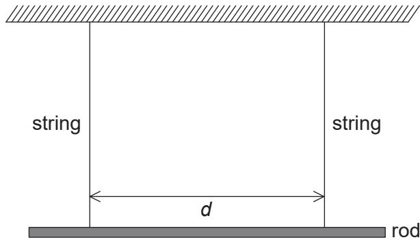
When the rod is displaced by a small angle and then released, simple harmonic oscillations take place in a horizontal plane.
