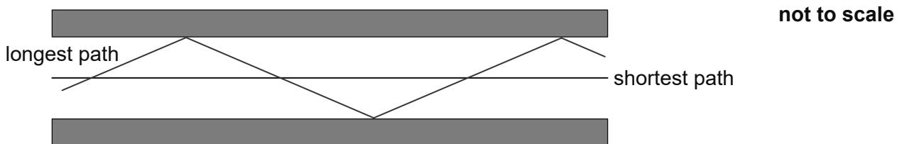
For the longest path the rays are incident at the core-cladding boundary at an angle just slightly greater than the critical angle. The optic fibre has a length of 12 km.
